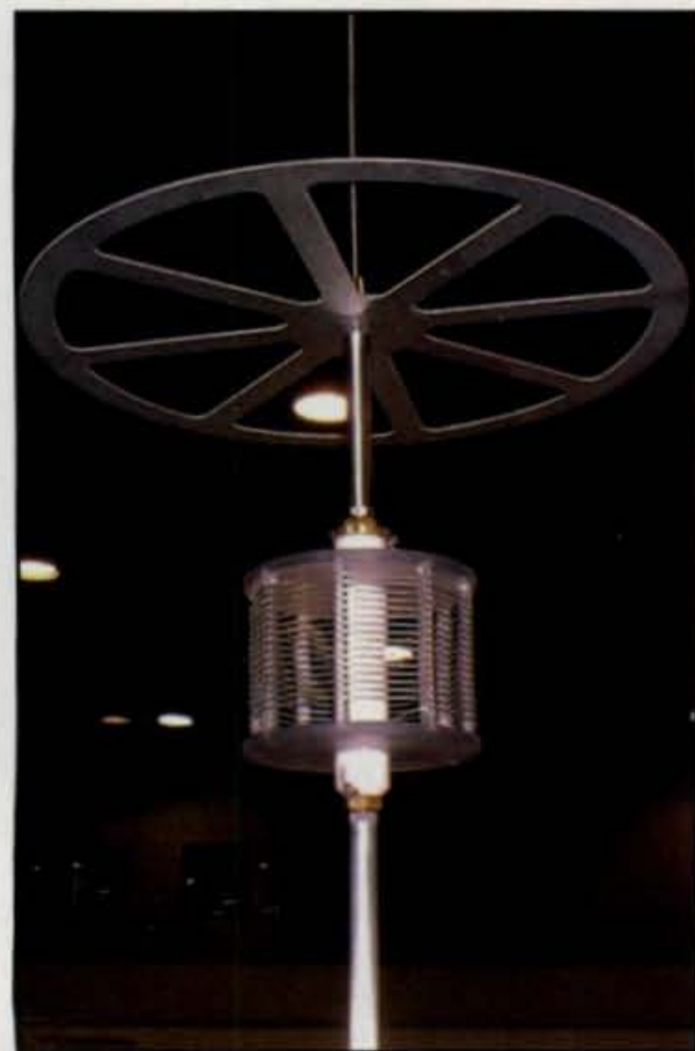
Photo B— Loading coils.
